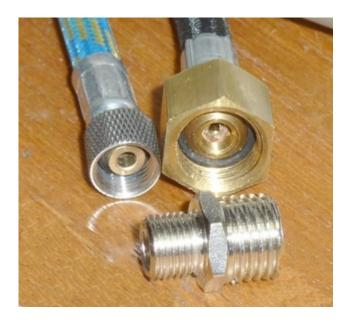
Here is the adaptor in position. At first the joint leaked air so I had to fit an O-ring into the 1/4" connector as you see in the above picture. The one that fitted best from the set that I had was 13mm outside diameter and 1.5mm rubber diameter. It worked perfectly.
